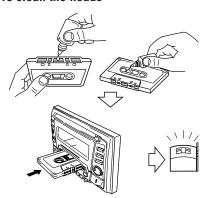
Clean the heads after every 10 hours of use using a wet-type head cleaning tape (available at an audio store).
